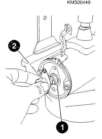
Checking armature braking torque
